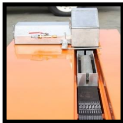
V core holder in automatic feed slot (nylon belt drive shown)
