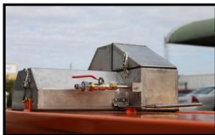
Blade cover housing with lock down latches and water tap
